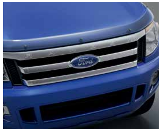
Bonnet Protector – Helps prevent scratches and stone chips on the bonnet.
