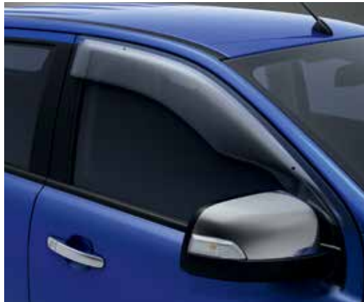
Weather Shield – The bubble weather accessory helps deflect wind and rain from the inside of the vehicle while driving with the window open.
