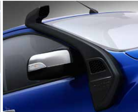
Snorkel – This tough and stylish UV resistant snorkel has been designed to deliver high volumes of the coolest and cleanest air possible to the engine.
